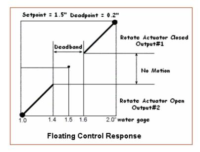
Simple floating controllers are quite satisfactory provided that the controlling thermostat in heating systems is able to sense quickly the effects of the corrective action it produces. The corrective action (movement of a valve or damper) always takes place at the same rate in simple floating control, irrespective of whether the deviation or error signal is large or small.
