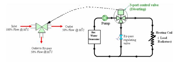
**Diverting Valve in Heating Applications**
