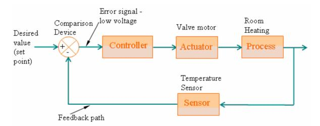
Heating System Control Loop Diagram
