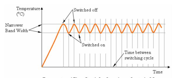
Temperature / Time Graph for Open Loop Control of Oven
