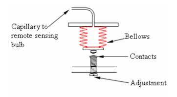
Sealed Bellows Temperature Sensor
