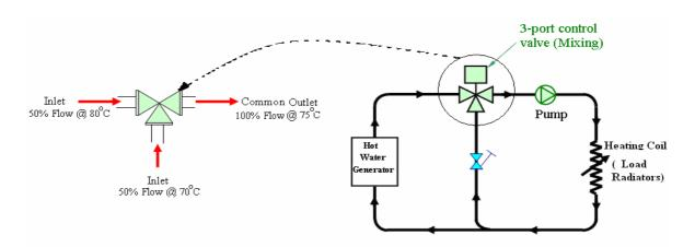
Mixing Valve in Heating Applications
