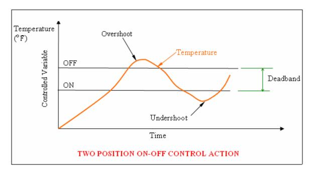
The response curve is always cycling between the two limits 'on' and 'off', and overshoot and undershoot occur in practice due to the thermal inertia of buildings and plants.
