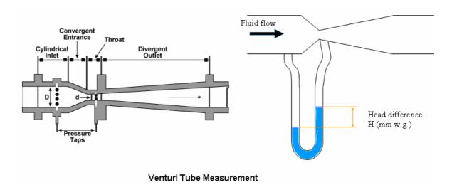
Venturi tubes exhibit a very low pressure loss compared to other differential pressure meters, but they are also the largest and most costly. Venturi tube applications are generally restricted to those requiring a low pressure drop and a high accuracy reading. They are widely used in large diameter pipes.
