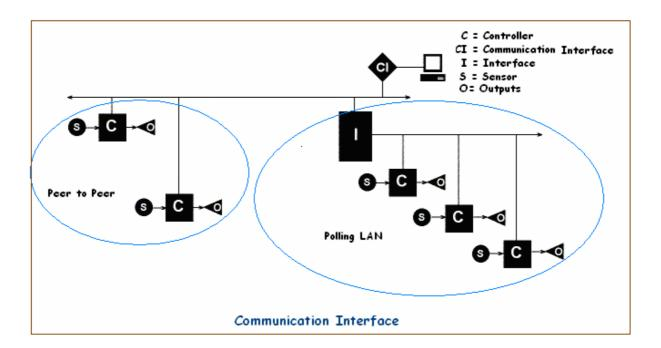
The interface device manages communication between the polling LAN controllers and the higher levels in the system architecture.
