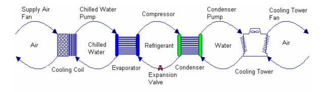
Chilled Water System With Water Cooled Condenser
