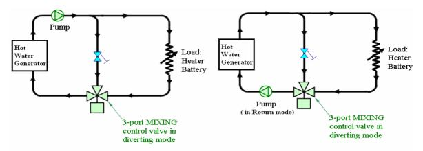
3 - Port Mixing Valve as Diverting Valve Application
